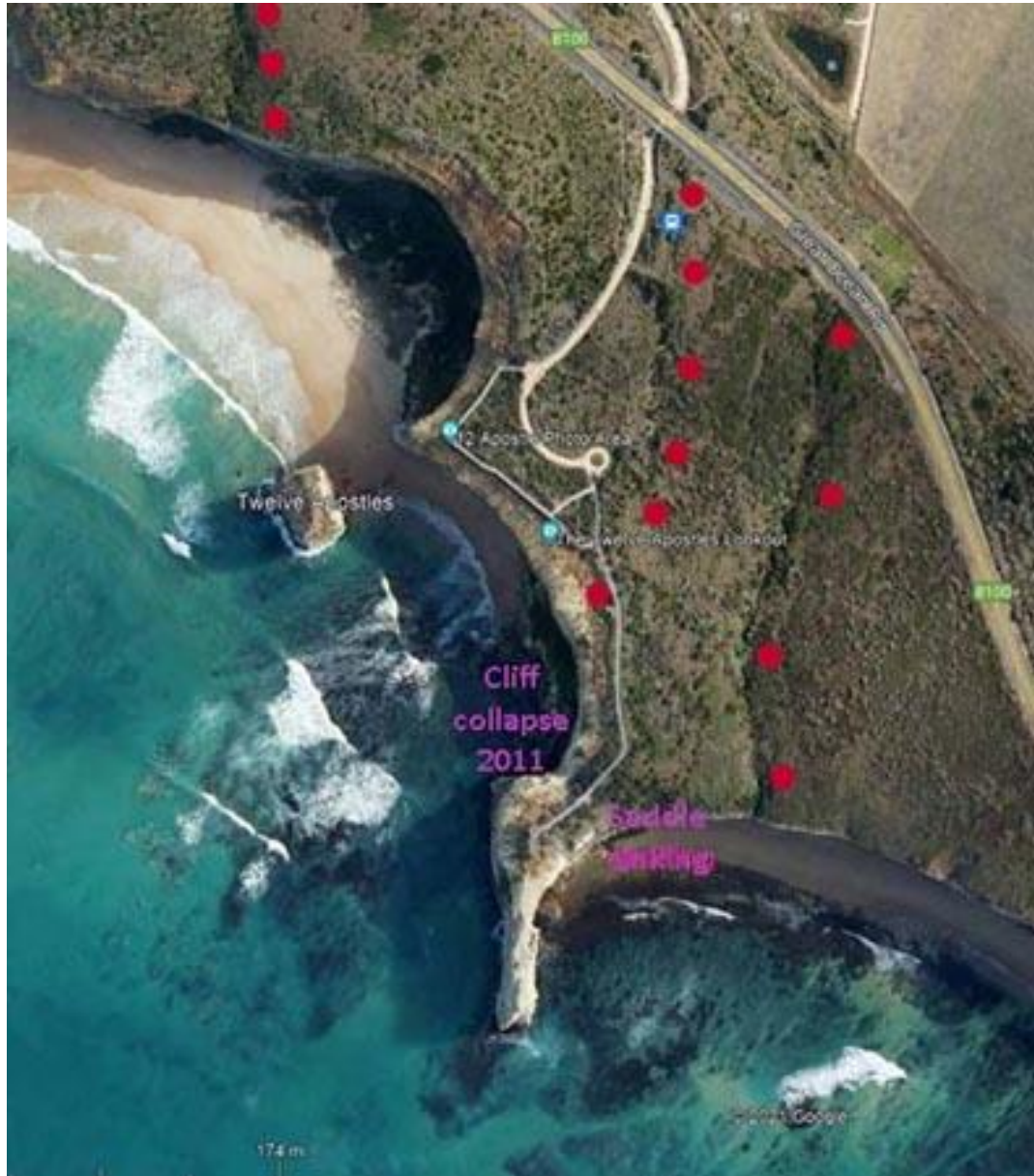
Photo: Google Earth. Red dots show drainage channels. The Saddle & the Castle Rock promontory is eroding
