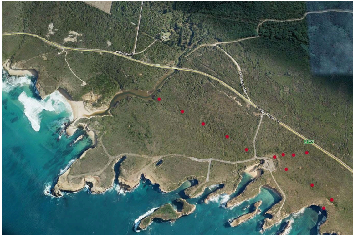
Photo: Google Earth – red dots show underground caverns and lineations which run through to Sherbrooke River under the Loch Ard Gorge car park.
